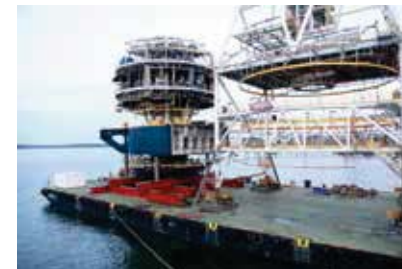
OSX-3 Turret Fabrication of a turret for OSX-3 FPSO Client : Sofec Inc Weight : 3,500 MT Location : Campos Basin, Offshore Brazil
